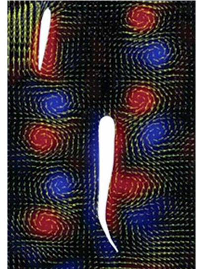
Hydrodynamic flow patterns using particle image velocimetry. Photo courtesy of the Lauder lab
